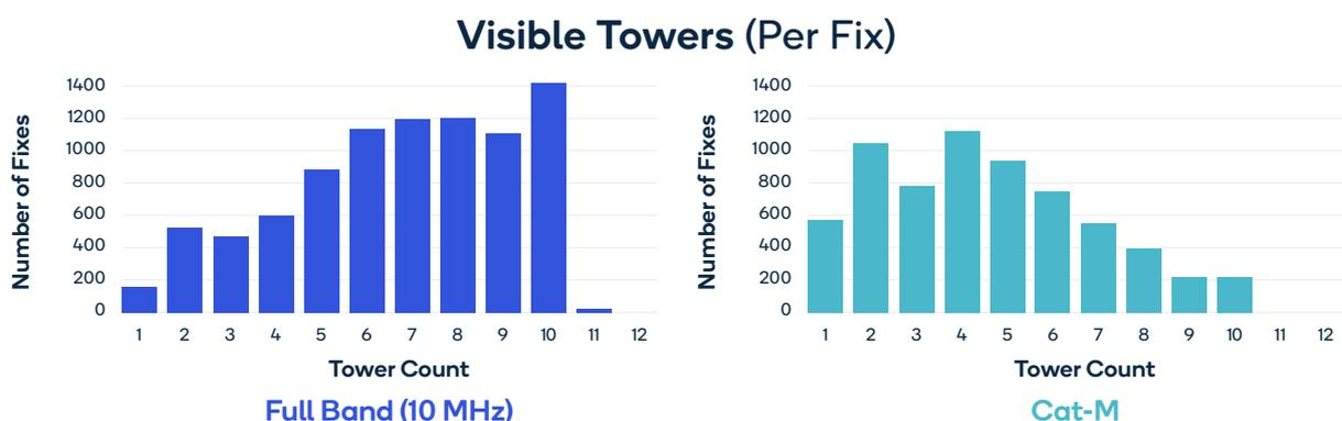
**Figure 2: Towers detected, 10 MHz channel vs. Cat-M device**
